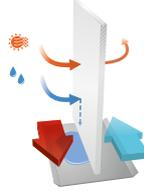
o The **KOMFORT Ultra L 250-E S12 (white)** unit is equipped with an enthalpy plate cross-flow heat exchanger for energy (heat and humidity) recovery. Due to humidity recovery condensate is not generated in the enthalpy heat exchanger.
